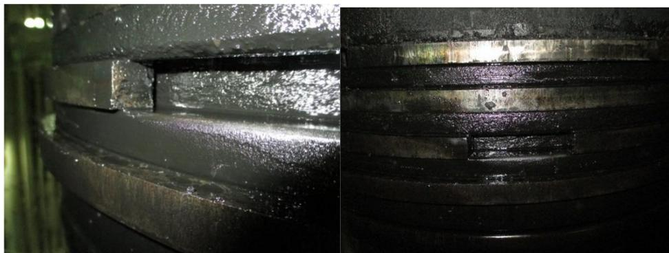
**Figure 2.** Damaged piston rings
