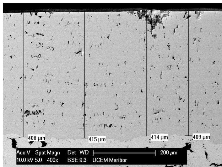
**Figure 10.** Thickness of the Cr-Al<sub>2</sub>O<sub>3</sub> coating on the Top ring GGV examined by electronic microscope (SEM) [21]
