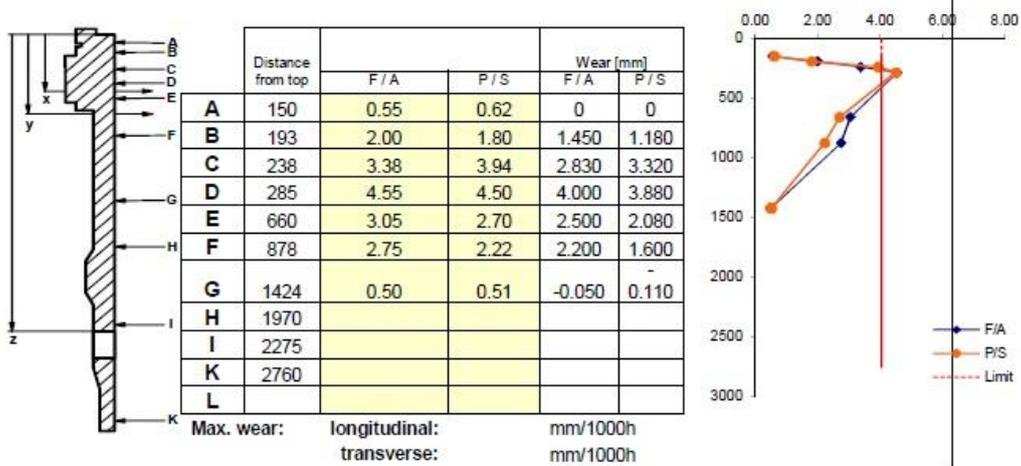
Figure 3. Measured wear of the cylinder liner
