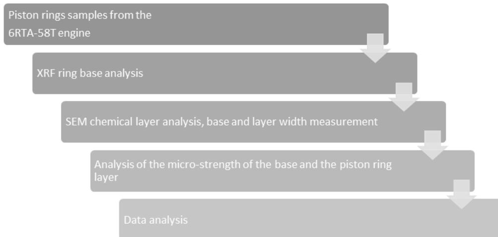
**Figure 6.** Methodology of analysing the piston ring samples
