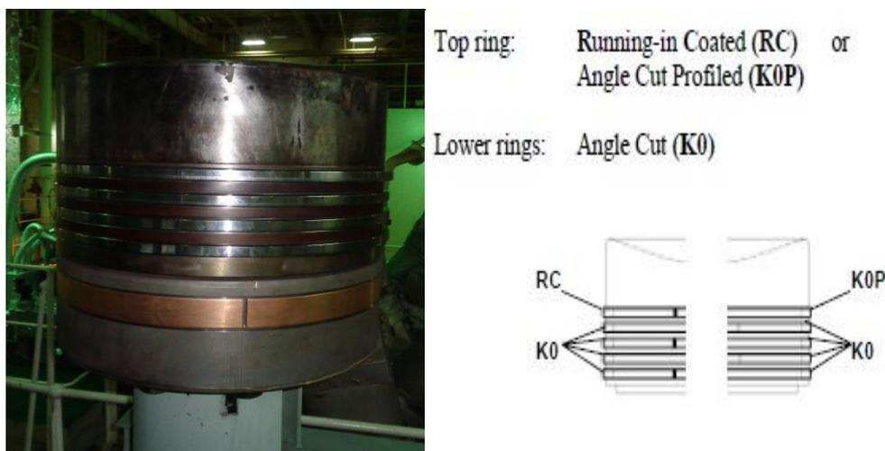
Figure 1. Design and configuration of the piston rings
