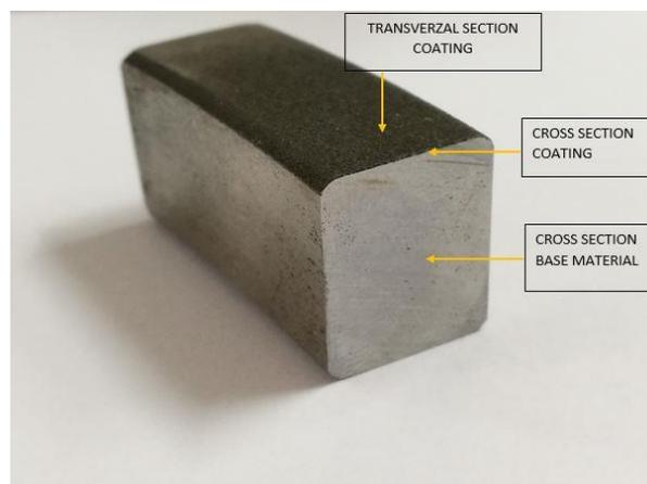
**Figure 13.** Points of measurement for Vickers micro-hardness [21]
