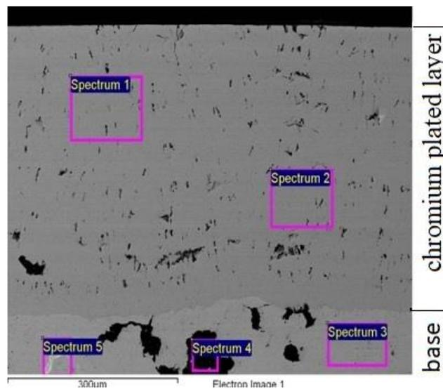
**Figure 9.** Polished section of composite coating Cr-Al<sub>2</sub>O<sub>3</sub> by piston ring producer Goetz [21]
