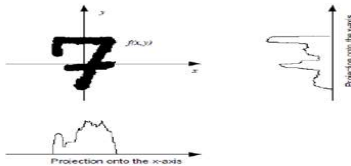
Fig 2. Radon Transform Horizontal & Vertical Projection View
