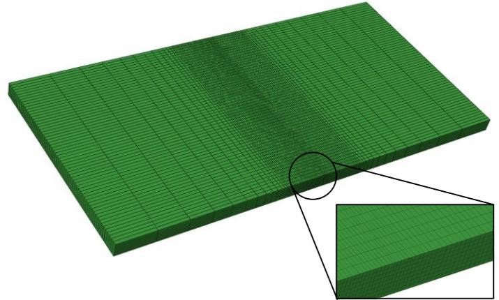
**Fig. 5.** Finite element mesh of two butt-welded plates
