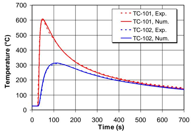
**Fig. 6.** Temperature-time histories at nodes TC-101 and TC-102
