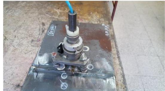
**Fig. 4.** Measurement of residual stresses
