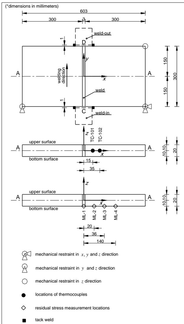
**Fig. 2.** Geometry of two butt-welded plates
