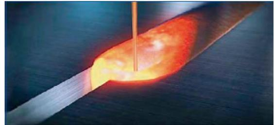
**Fig. 1.** Buried arc process [13]
