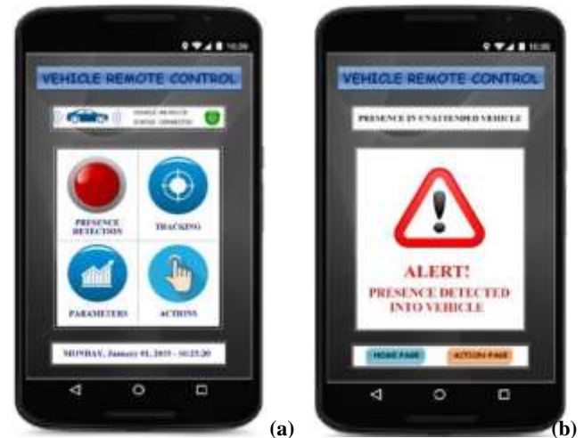
Fig. 15. Application's main dashboard (a) and alarm dashboard (b).
