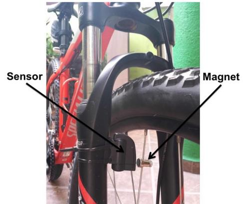
Fig. 2. Magnet on a cycle wheel spoke and sensor mounted on the right suspension fork measure when the wheel makes a spin. [10]
