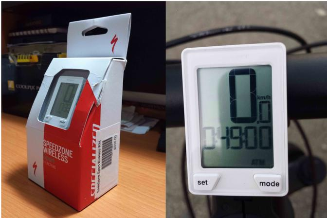
Fig. 1. Cycle computer (Specialized Speed Zone Sport Wireless) receives data from a sensor mounted on the suspension fork. [10]
