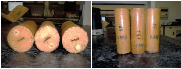
Figure 5 Test samples of polymer grouting materials
