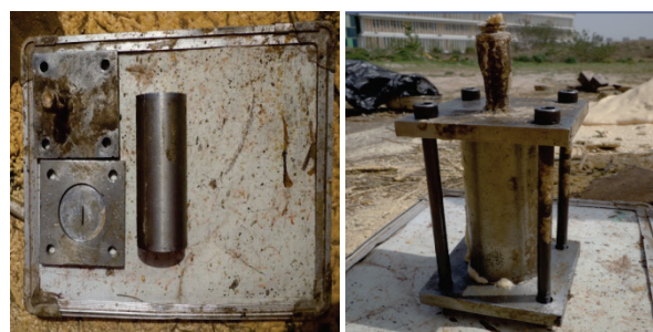
Figure 3 The specific mould of the bender elements samples
