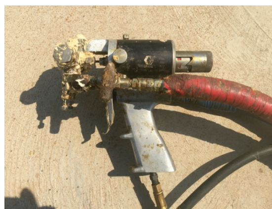
Figure 4 The grouting gun of polymer materials
