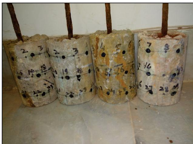
Figure 1 Samples for determination of corrosion potential.
