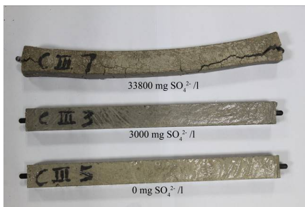
Figure 1. Appearance of the mortars after immersion in the Na 2 SO 4 solutions for 450 days.
