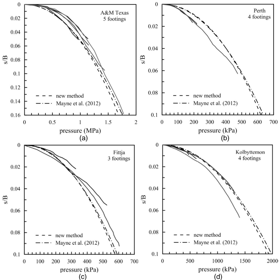
Figure 7. Normalized settlement vs. applied footing pressure for the four locations
