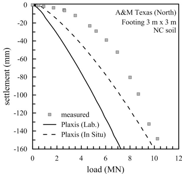
Figure 1. Measured and calculated settlements of A&M Texas 3 m x 3 m North footing; calculated settlements are with laboratory and in situ parameters from Table 1 for normally consolidated soil; measured settlements from Briaud and Gibbens (1997)
