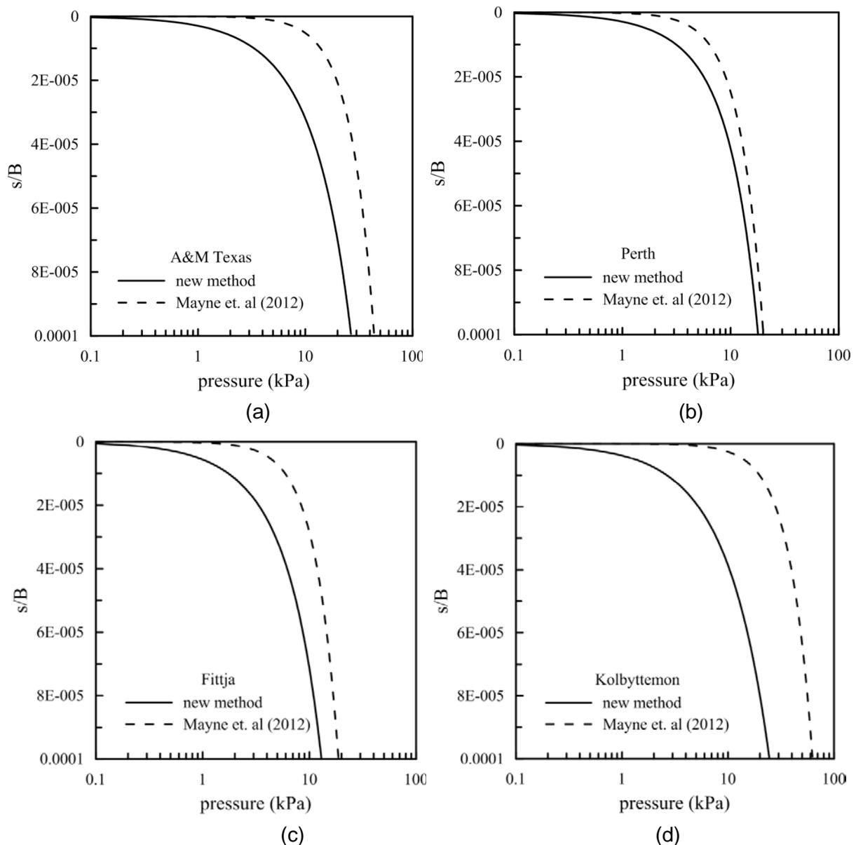
Figure 8. Normalized settlement vs. applied footing pressure at very small strains for the four locations
