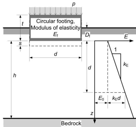
Figure 4. Notations related to the Mayne and Poulos (1999) method for calculation of settlements of a flexible circular footing embedded in the Gibson type of soil (Gibson, 1967)
