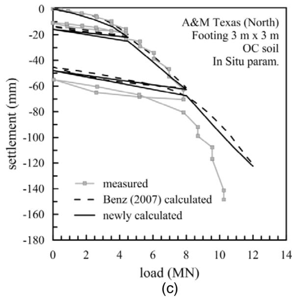
Figure 2. Measured and calculated settlements of A&M Texas 3 m x 3 m North footing: (a) normally consolidated soil (NC), laboratory parameters; (b) overconsolidated soil (OC), laboratory parameters; (c) overconsolidated soil (OC), in situ parameters; measured settlements from Briaud and Gibbens (1997)
