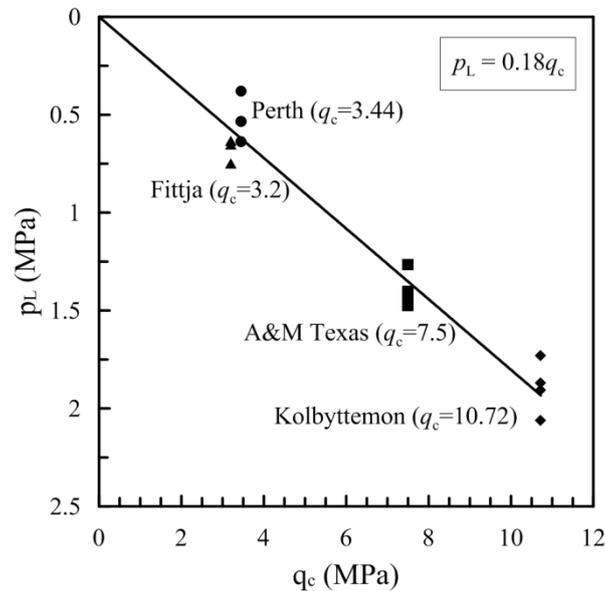
Figure 6.  $p_L$  and  $q_c$  for all 16 footings ( $q_c$  values taken from Mayne et al., 2012)
