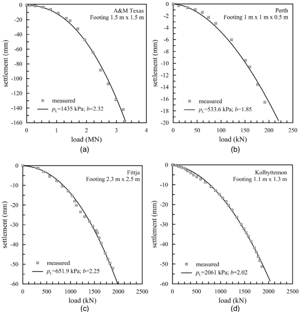
Figure 5. Measured data and fitted curve for one footing from each location:  $p_L$  and  $b$  from Table 3
