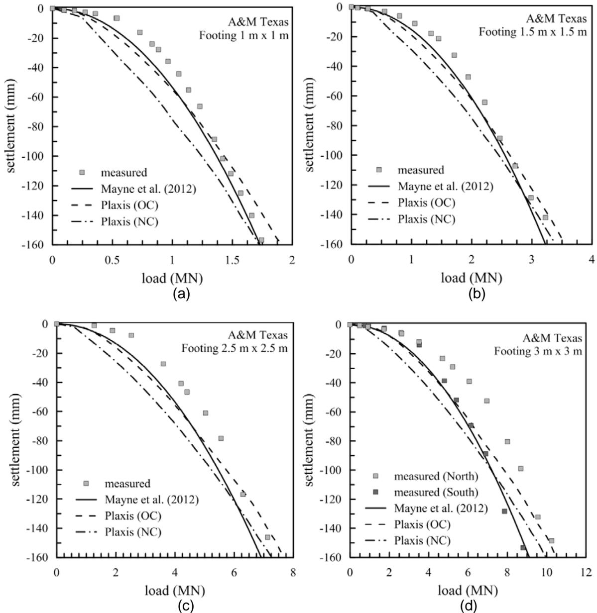
Figure 3. Measured and calculated settlements for all A&M Texas footings; measured settlements from Briaud and Gibbens (1997); calculated by Plaxis 2D for overconsolidated soil through calibration with Mayne et al. (2012); calculated by Plaxis 2D for normally consolidated soil
