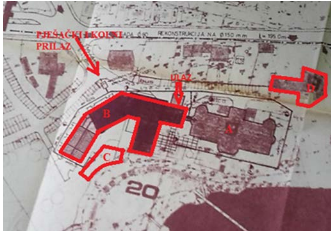
Figure 5. Layout plan from the extension design, 1983. (A- historical part of the hotel; B, C extension, D added outbuilding). Rijeka projekt d.o.o. 1985.
