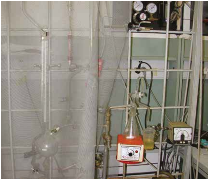
Figure 7. Extraction by partially degassing with mercury, high risk-low efficiency
