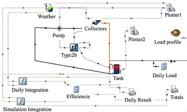
Figure 8 Simulation model for the solar hot water system
