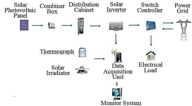
Figure 9 System schematic of the operating solar photovoltaic system
