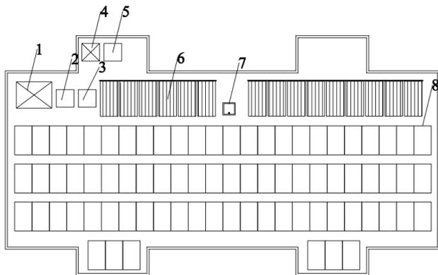
Figure 7 Roof plan for thermal collectors and photovoltaic panels: 1 - Electrical Cabinet, 2 - Solar Inverter, 3 - Photovoltaic Controller, 4 - Water tank, 5 - Heat Pump, 6 - Thermal Collector, 7 - Roof Access, 8 - Photovoltaic Panel
