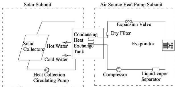
Figure 6 System schematic of the solar hot water system
