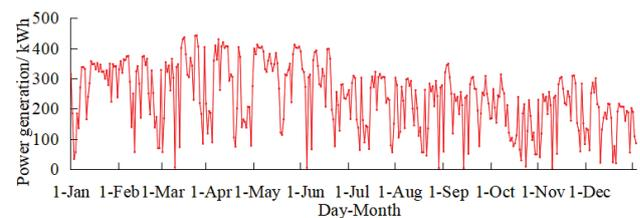
**Figure 13** Monitoring data of electricity generation of the solar photovoltaic system in one year
