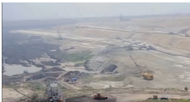
Figure 1 Open-pit coal mine with basic and auxiliary machinery and conveyor belts
