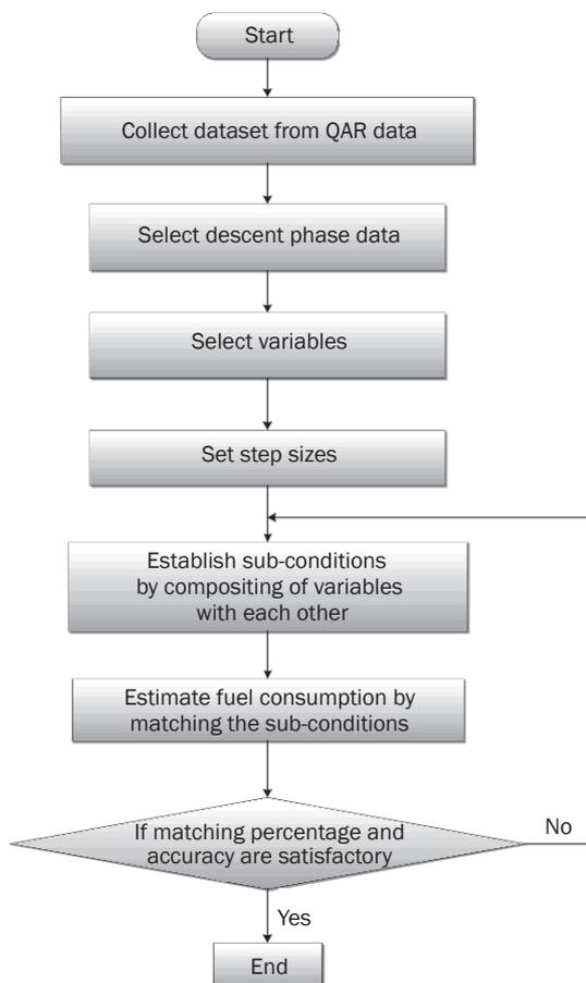
*Figure 1* – Illustration of sub-match method
