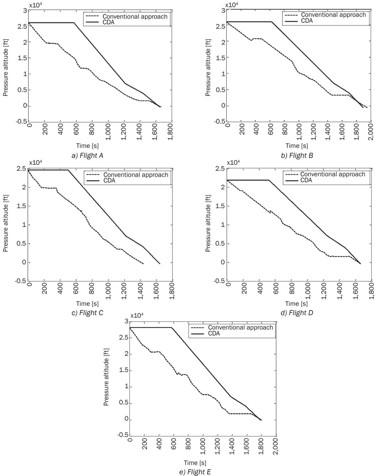
Figure 10 – Vertical trajectory profiles for A~E flights
