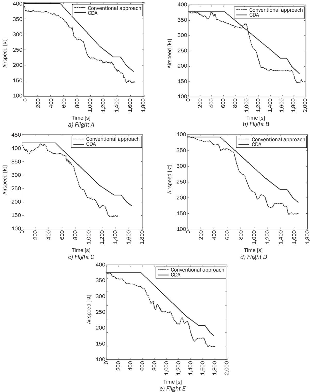
Figure 11 – Airspeed profiles for A~E flights
