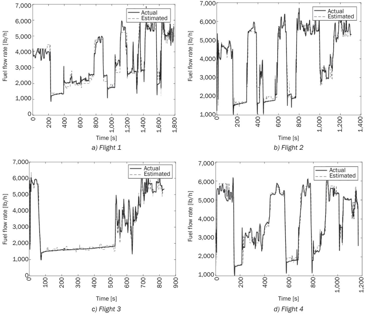
Figure 2 – Estimation of fuel flow rates for Boeing 737-800
