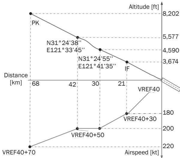
Figure 5 – Vertical trajectory and speed profiles of CDA procedure for runway 17L at Pudong International Airport
