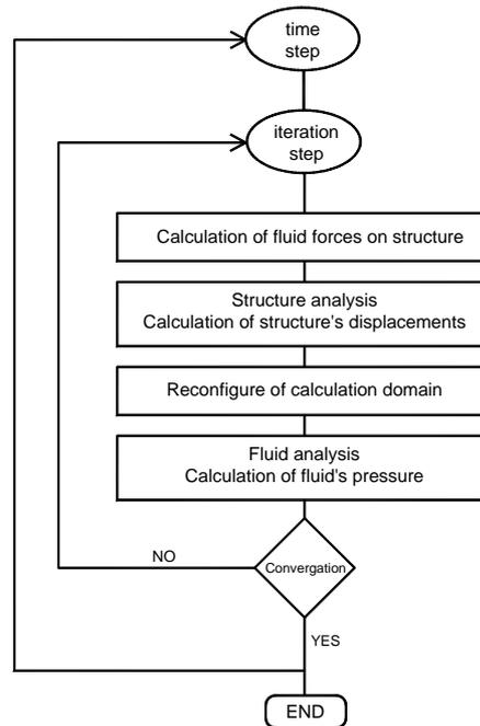
**Fig. 7** The solution scheme for the fluid-structure coupled problems analysis
