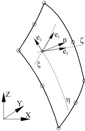
**Fig. 6** The fluid-structure interaction surface and unit norm
