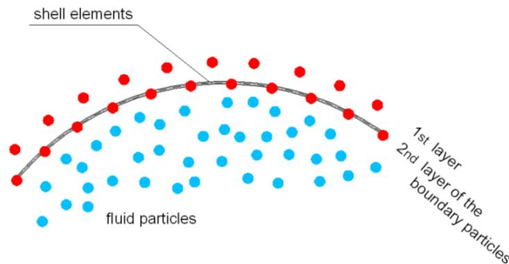
**Fig. 5** Virtual fluid particles on the interface
