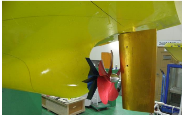
Fig. 15 Experimental setup for the self-propulsion test
