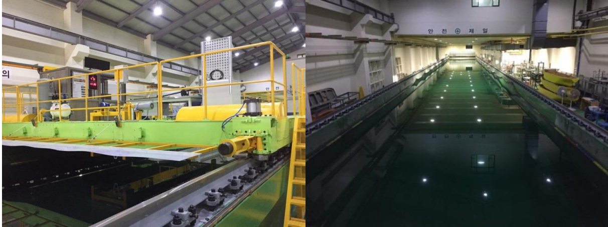
Fig. 13 Towing carriage and tank at PNU
