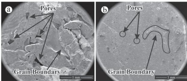
**Figure 6** SEM image of unreinforced Cu10Sn morphology (a) before sintering and (b) after sintering.
