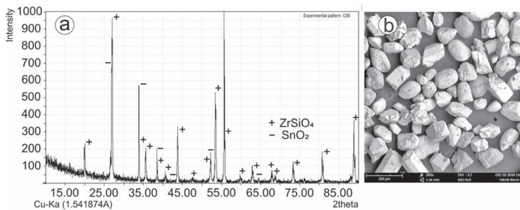
**Figure 1** (a) X-Ray Diffraction (XRD) pattern and (b) scanning electron microscope (SEM) Image of SnO<sub>2</sub> tailing sand.
