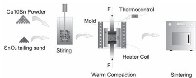
**Figure 2** Schematic diagram of the composite production process.
