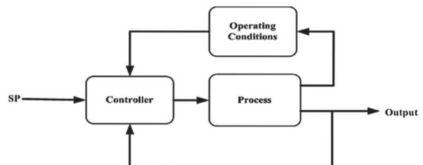
Figure 5. General block diagram of gain scheduled controller.
