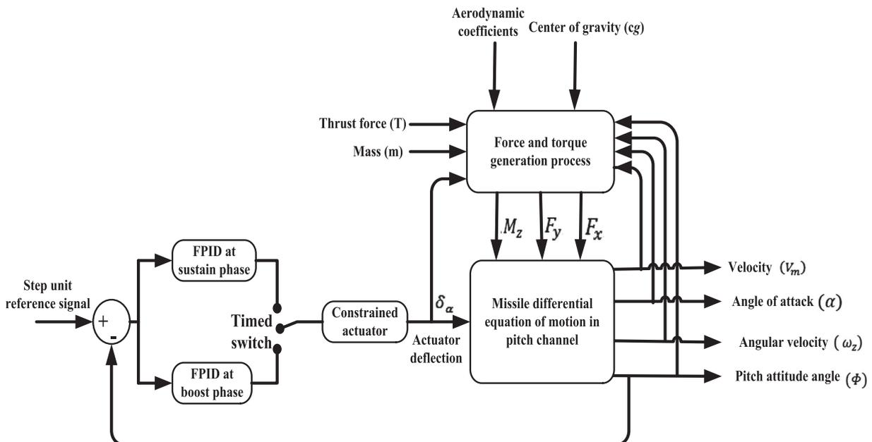
**Figure 14.** Block diagram of nonlinear dynamic system with *GSFPID* in pitch Channel.
