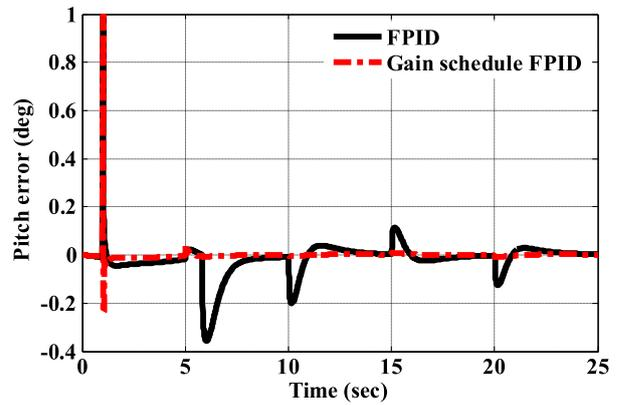
Figure 24. Pitch error comparison with wind effect.
