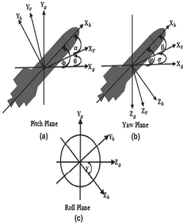
Figure 1. The angles between different coordinate systems.
