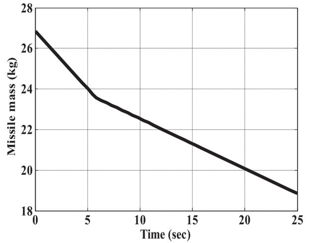
Figure 7. Missile body and variable propellant mass curve.
