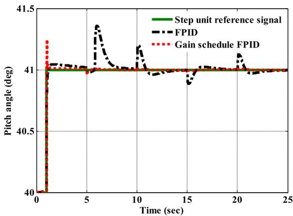
Figure 23. Pitch angle comparison with wind effect.
