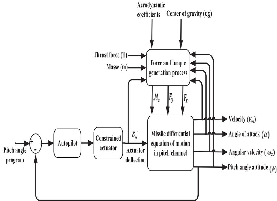
**Figure 3.** Block diagram of pitch angle attitude control.
