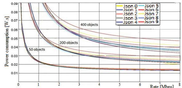
Figure 7 Comparative presentation of energy consumption depending on the speed of flow and amount of data
