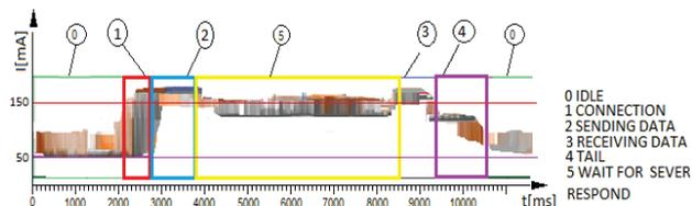
Figure 4 The results of measuring two REST profiles with increased server delay times
