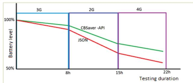
Figure 11 The results of comparative measuring of a CBSaver API and a classical JSON manner of transfer
