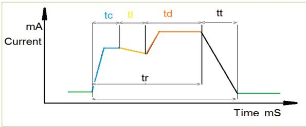
Figure 2 Segmented presentation of an energy profile of a REST request
