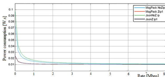
Figure 8 The relationship between the consumption of JSON and MsgPack schemes at different levels of compression
