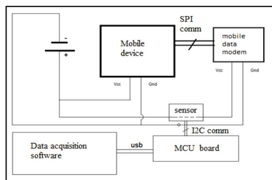
Figure 1 A schematic diagram of the measuring equipment
