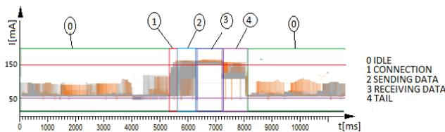
Figure 3 The results of measuring two REST profiles with marked segments
