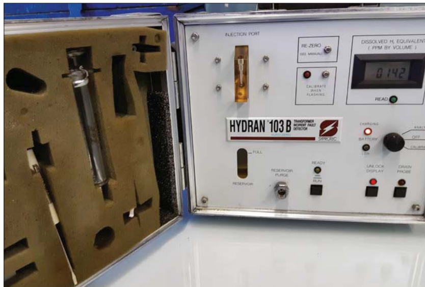
Figure 9. Portable device 103B, efficient, cheap and accurate device for DGA
