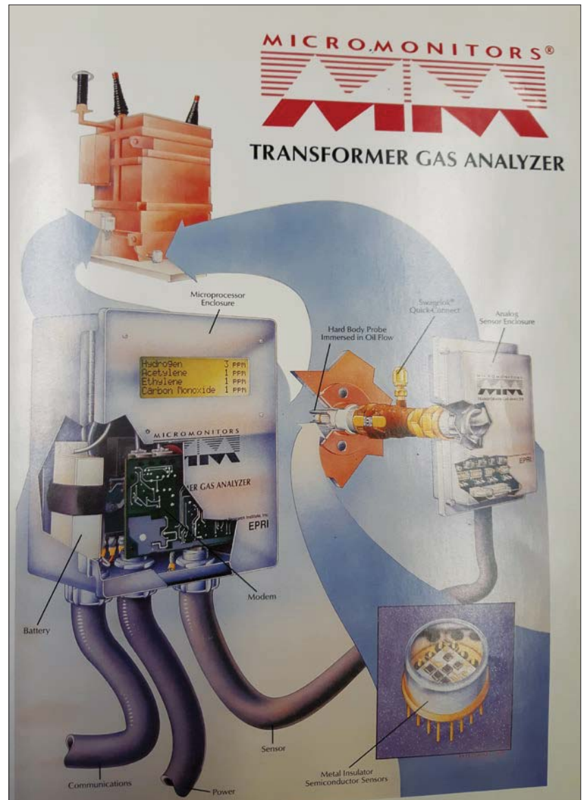
Figure 11. First attempt to directly measure gases in oil, despite the EPRI reputation, was not successful and the company that developed it in 1992, later known as SERVERON, adopted GC technology and, recently, switched to their version of PAS for DGA
