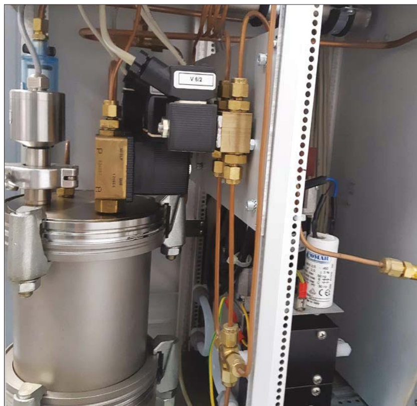
Figure 13. Two non-mercury vacuum extraction systems a) partial, b) a scheme of multi-stroke complete extraction; the present alternatives to previous Torricelli, Toppler and McCleod devices
