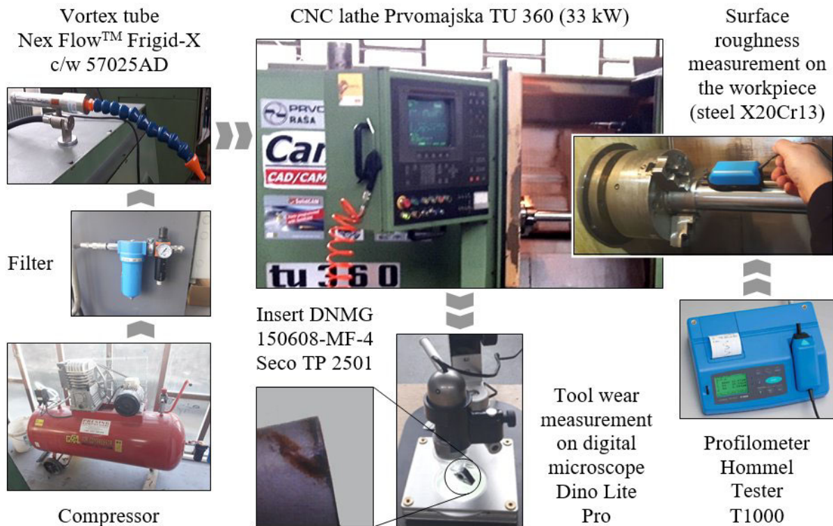
Fig. 2 Experimental configuration for the testing of machinability
