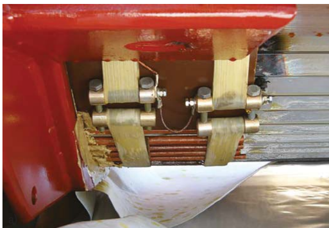
Figure 7. a) and b) Improper earthing induces an abrupt gas increase three years after energizing
