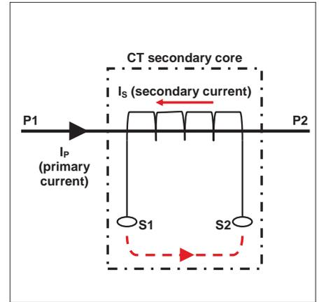
Figure 9. Current transformer connection
