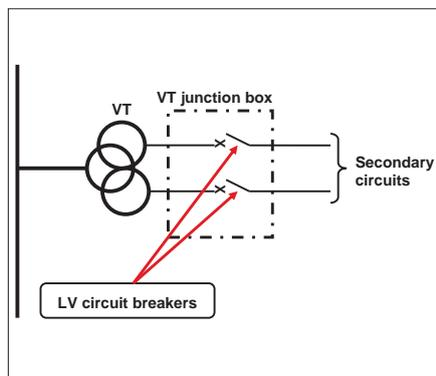
Figure 8. Voltage transformer junction box
