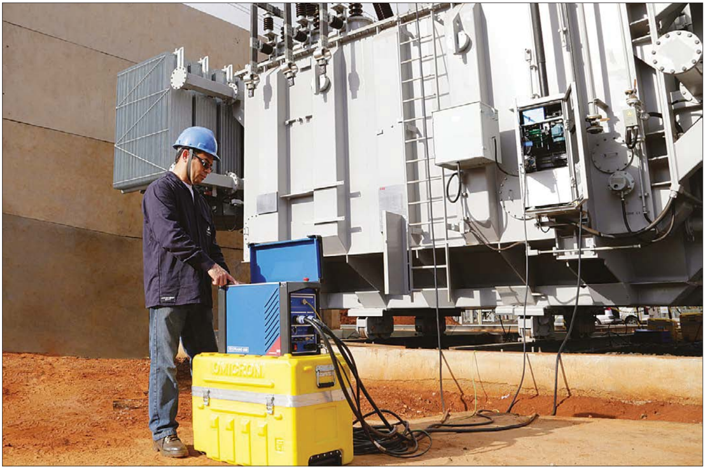
Figure 2. Using a three-phase test system can significantly reduce the effort for rewiring between the individual power transformer tests
