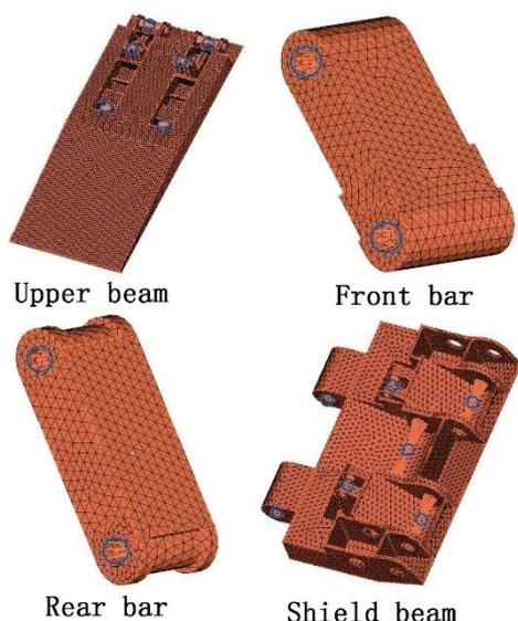
Figure 5 Flexible grid meshing of main structural components
