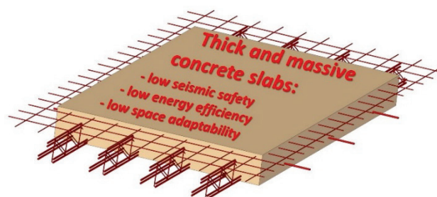
Figure 7 Illustration of the negative aspects of thick and heavy concrete floor slabs which hinder adaptability, energy efficiency and seismic safety of residential buildings
