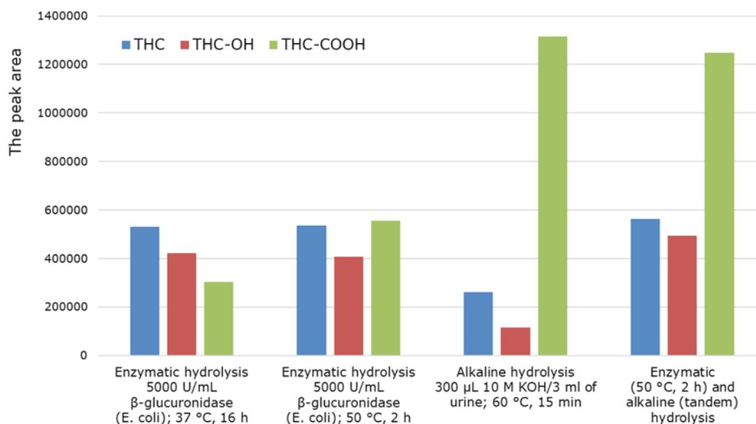
**Figure 1** Comparison of different types of hydrolysis for cleavage of conjugates THC, THC-OH, and THC-COOH from 24-hour rat urine (pooled sample of five rats that received a single dose of 20 mg of THC/kg bw orally)
