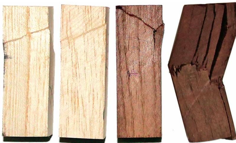
**Figure 3** Specimens after the completion of compression strength test
