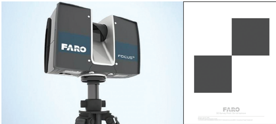
Figure 3 FARO 150 S 3D laser scanner (left) and paper checkerboard (right)
