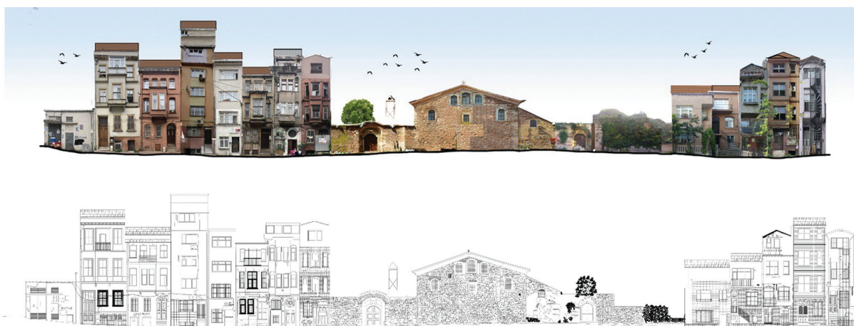
Figure 5 Post production orthographic-photograph and Autocad drawings for the west facade of Murat Molla Street.
