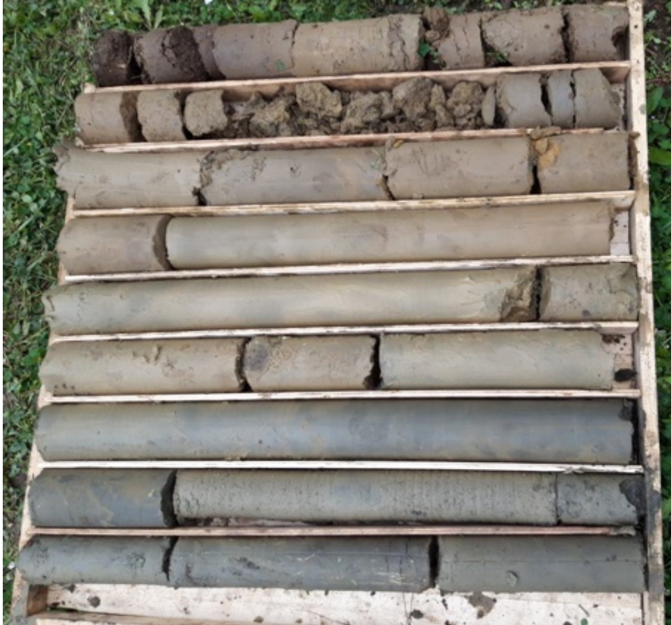
Figure 1. Drilled cores from the borehole NB-1
