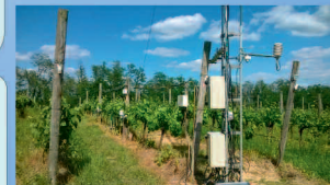
Picture shows instruments in first 2 meters. For characterizing the microclimate the relative humidity and temperature, wind speed and direction, UV, leaf wetness and leaf temperature were measured inside the cordon rows among the leaves. Temperature, relative humidity and wind speed gradient have been also measured above the plants.
