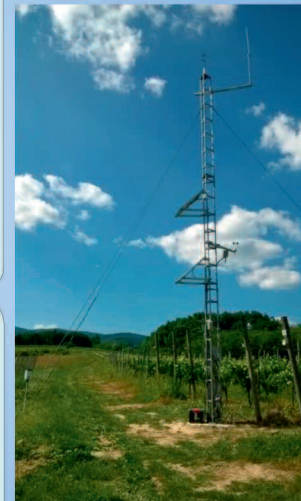
Meteorological tower (10 m) with solar panels, radiation, temp, humidity and wind measurements
