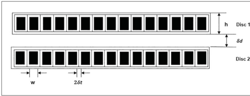
Figure 5a. Representation of transformer winding (two disc)
