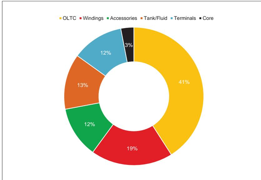
Figure 1. Survey of faults in transformer [3]
