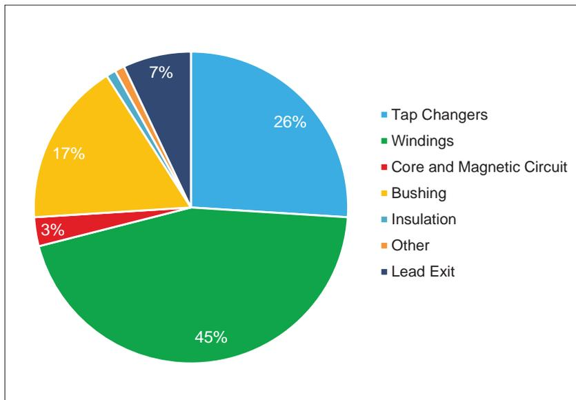
Figure 2. CIGRE failure statistics [4]
