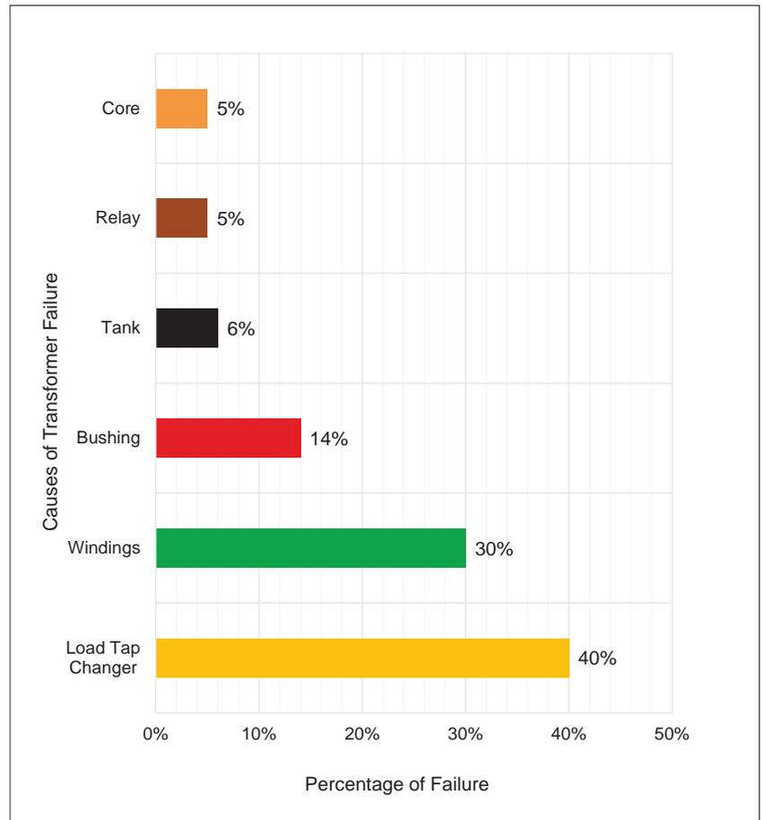
Figure 3. Causes of transformer failure [5]
