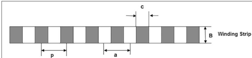
Figure 5b. Representation of winding strip used for inductance calculation
