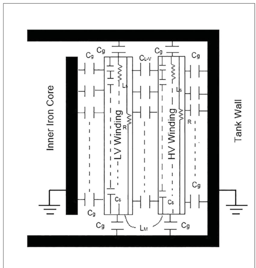
Figure 4. Transformer assembly schematic diagram
