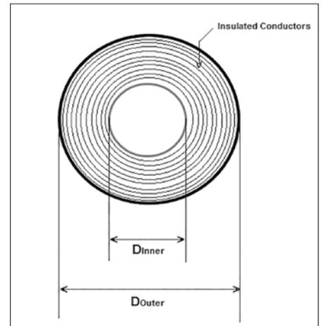
Figure 6. Schematic of transformer winding (top view)
