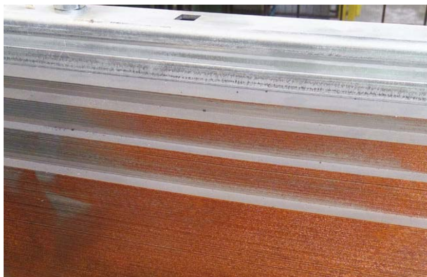
Figure 1. Rust on the core lamination edges
