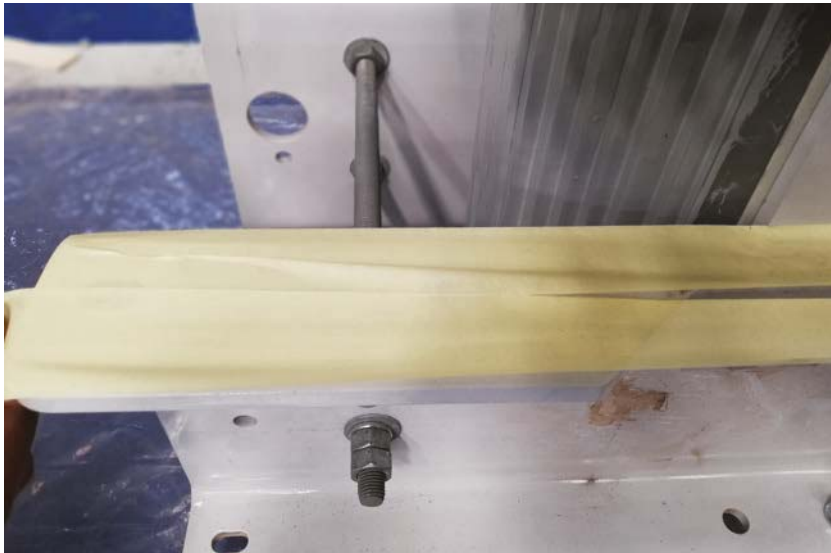
Figure 6. Areas that will not be painted, such as clamps or core leg plates should be isolated by using the paint masking tape
