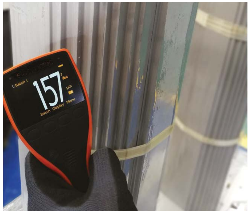
Figure 9. Measuring the coating thickness using a digital coating thickness gauge
