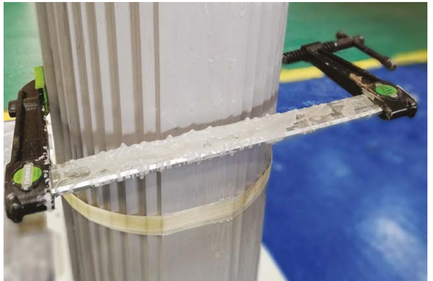
Figure 5. Adhesive tapes or any fixtures used for binding core laminations should be removed after stacking process is completed
