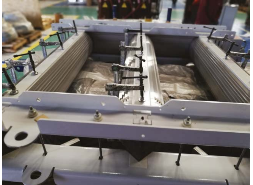
Figure 4. Bonding fixtures along the height of the limbs and bolts should be firmly tightened before the core is taken off the stacking rig
