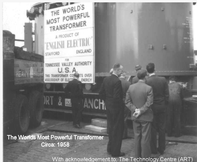
Figure 4. 1958 - The world's most powerful transformer at that time: 345 MVA 22.5 / 160 kV. Reference: New Scientist, April 2nd 1959
