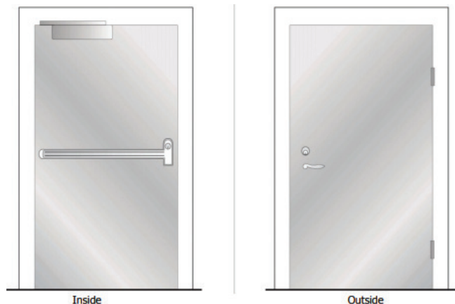
Slika 2 – Jednokrnlina vatrootporna vrata (izvor: Panic & emergency exit devices CFFA-E Guideline No 2:2013 F)
