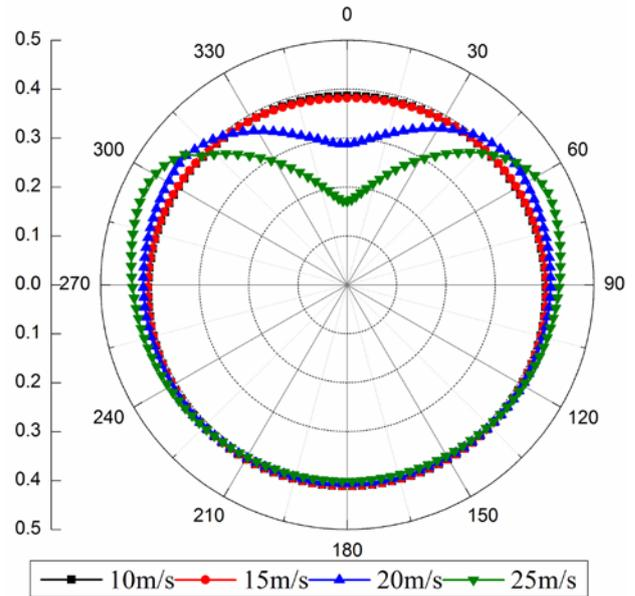
Figure 4. Deformation of pipeline under different impact velocities
