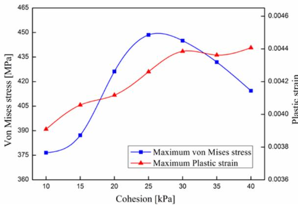
Figure 11. Stress and strain under different cohesions
