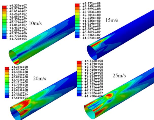
Figure 3. Von Mises stress under different impact velocities
