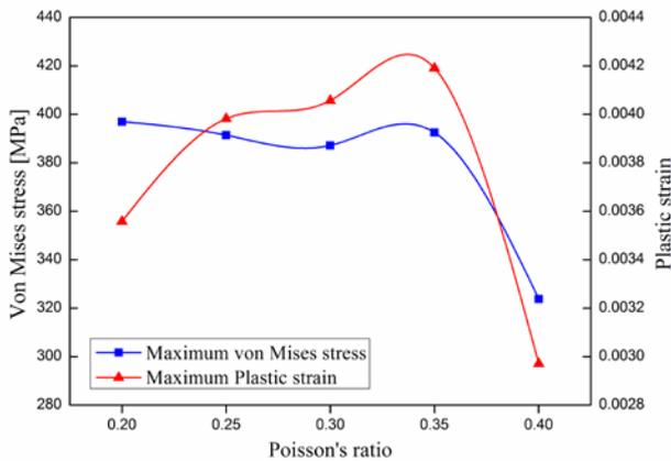
Figure 8. Maximum stress and plastic strain under different Poisson's ratios when  $v=15\text{m/s}$
