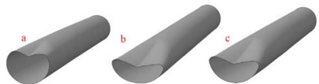
Figure 2. Deformation process of the buried pipeline
