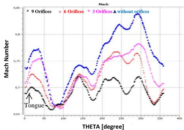
Figure 13. Variation in the number of Mach as a function of the azimuth angle in the mean radius line around the rotor entrance ( $P0^* = 1.445 \text{ bar}$ ).
