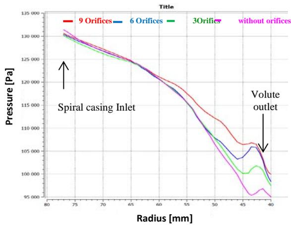
Figure 6. Variation of the static pressure along the average stream line according to the radial position ( $P0^* = 1,445 \text{ bar}$ )
