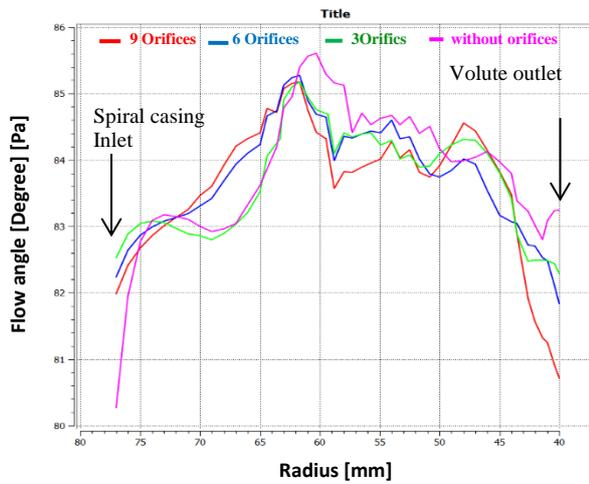
Figure 10. Variation of the Flow angle along the average stream line according to the radial position ( $P0^* = 1,445 \text{ bar}$ )
