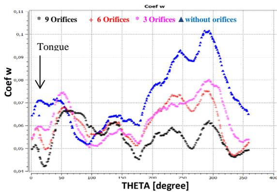
Figure 15. Variation of the total pressure loss coefficient as a function of the azimuthal angle in the mean radius line around the rotor entrance ( $P0^* = 1.445 \text{ bar}$ )
