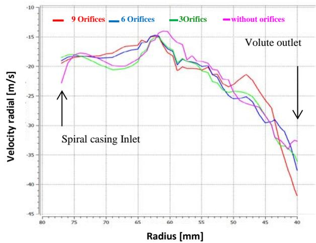
Figure 9. Variation of the radial velocity along the average stream line according to the radial position ( $P0^* = 1,445 \text{ bar}$ )
