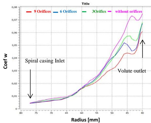
Figure 8. Variation of the total pressure loss coefficient along the average stream line according to the radial position ( $P0^* = 1.445 \text{ bar}$ )
