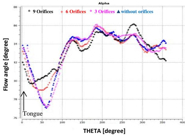
Figure. 14: Variation of flow angle as a function of the azimuthal angle in the mean radius line around the rotor entrance ( $P0^* = 1,445 \text{ bar}$ )
