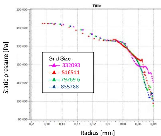
Figure 4. Grid solution independency
