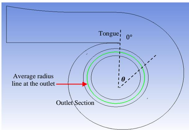
Figure 11. The average radius line at the outlet of the volute
