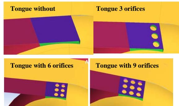
Figure 2. Different configurations of the tongues
