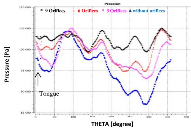
Figure 12. Variation in the Pressure as a function of the azimuth angle in the mean radius line around the rotor entrance ( $P0^* = 1.445 \text{ bar}$ )
