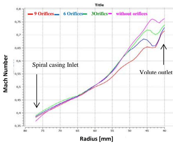
Figure 7. Variation of the Mach number along the average stream line according to the radial position ( $P0^* = 1.445 \text{ bar}$ )
