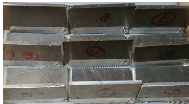
Figure 4. Dissimilar thickness friction stir corner joints.
