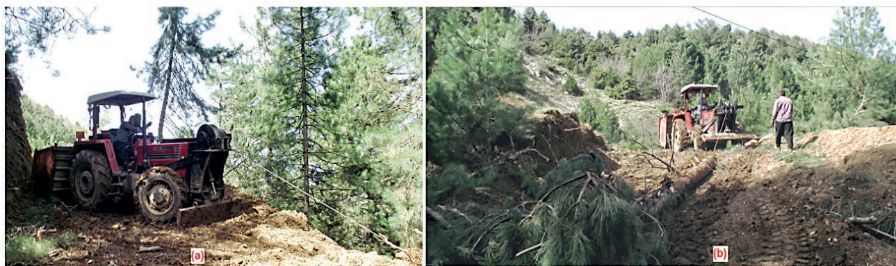
Figure 2. Timber extraction: uphill winching (a) and skidding backward on skid rail (b)
