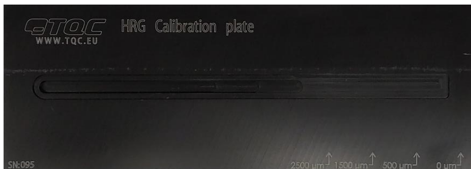
Fig. 5 Calibration plate of hull roughness gauge(DC-9000)
