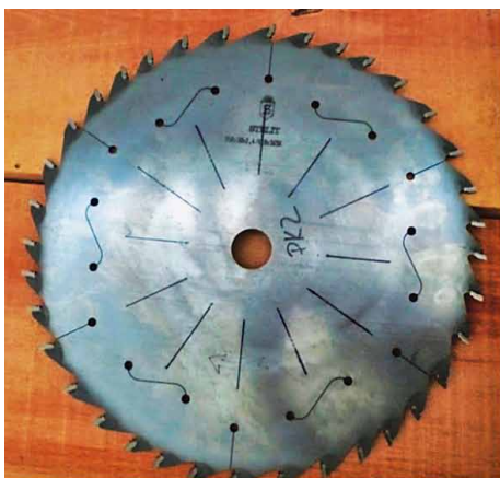
Figure 3 Circular saw blade 2 with irregular tooth pitch and body with dilatation gaps (Svoreň et al. , 2013)
