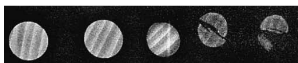
Figure 14 Radiographic images for cylindrical samples with approximately 20 mm of diameter and 5 mm height, after pyrolysis at 500^\circ\text{C} . From left to right: 30 s, 60 s, 90 s, 120 s and 150 s
