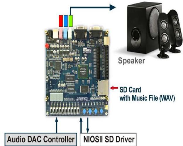
Fig. 5. The setup for the implemented test.
