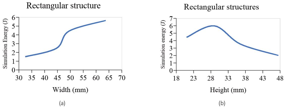
Figure 12. Simulation energy of rectangular structure by varying (a) width (b) height
