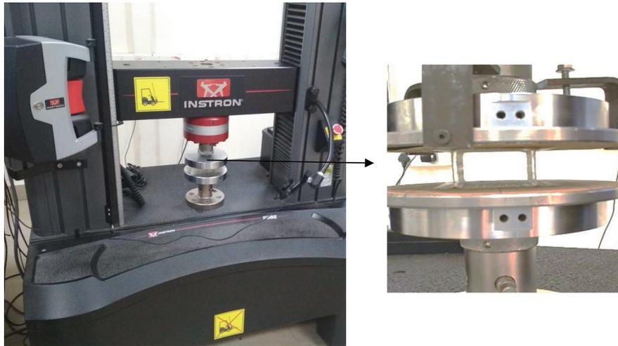
Figure 3. Experimentation setup for the compression test
