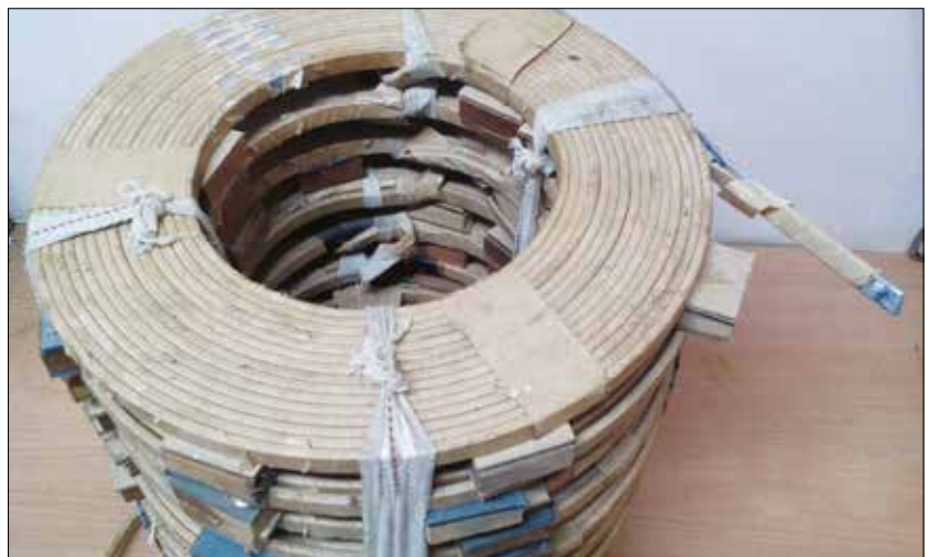
Figure 5. Continuous disc winding
