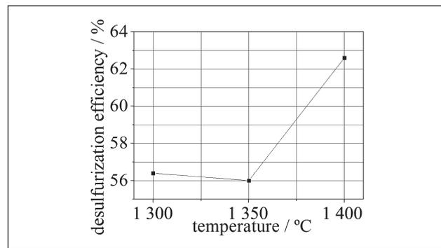
**Figure 4** Effect of temperature on desulfurization efficiency at current of 1 A
