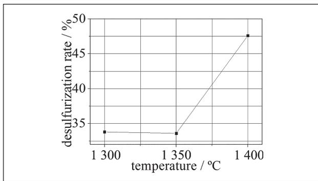
**Figure 3** Effect of temperature on desulfurization rate at current of 1 A
