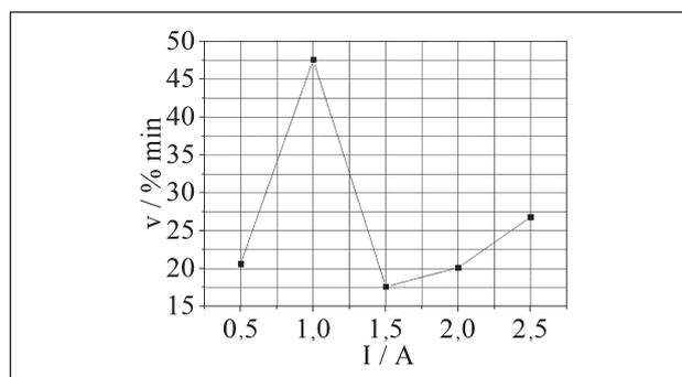
Figure 2 Effect of current on desulfurization rate at temperature of 1 400 °C
