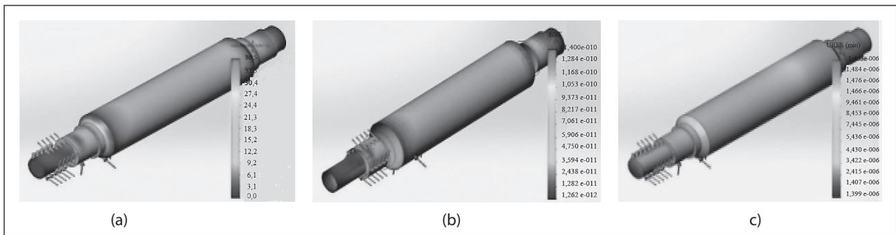
**Figure 5** The distribution of equivalent stresses (a) and deformations (b), as well as the total displacements (c) in the rollers during the transportation of the strips in a roller conveyor with lower air pressure.
