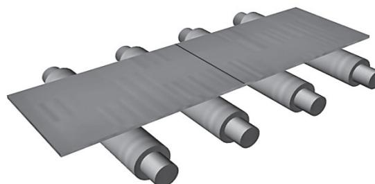
Figure 1 Force impacts at sheet shape control.
