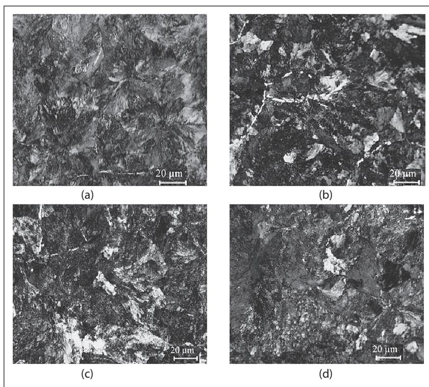
**Figure 4** The microstructure of 60C2XA steel after austenitization at 850 °C with a holding time of 1 h and subsequent hot deformation at temperatures of 700 and 800 °C and cooling for 3 and 6 s; (a) sediment at 700 °C and cooling 3 s; (b) sediment at 700 °C and cooling 6 s; (c) sediment at 800 °C and cooling 3 s; (d) sediment at 800 °C and cooling 6 s.
