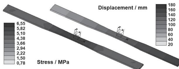
Figure 5 Belt conveyor static analysis results
