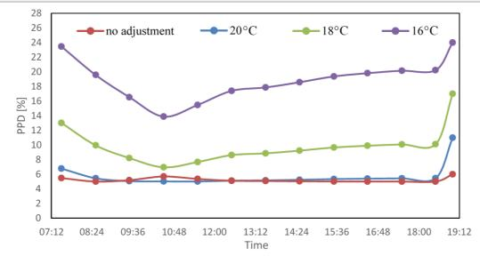
Figure 17. PPD around the heated chair when the setpoint was adjusted to 20, 18 and 16  $^\circ C$  (February 20<sup>th</sup>)
