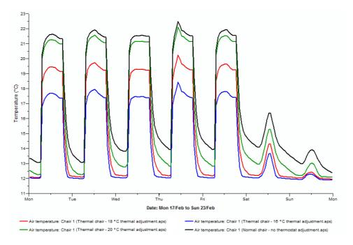
Figure 16. Air temperature results around the heated chair when the setpoint was adjusted to 20, 18 and 16 °C (17<sup>th</sup>-23<sup>rd</sup> February)
