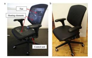
Figure 2. APCS device (a) and heating elements and fan installed on mesh thermal chair (b) covered thermal chair [32]
