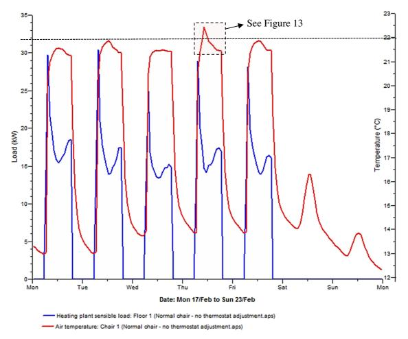
Figure 12. Air temperature results around the non heated chair and predicted heating load (17<sup>th</sup>-23<sup>rd</sup> February)
