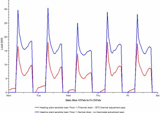
Figure 19. Hourly heating energy demand for the non heated chair and thermal chair with thermostat adjustment (17<sup>th</sup>-21<sup>st</sup> February)
