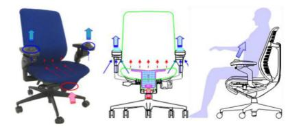
Figure 3. Airflow though the arm rest and seat of the cool chair [43]
