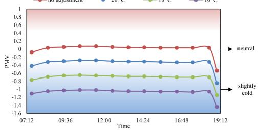
Figure 15. PMV around the non heated chair when the setpoint was adjusted to 20, 18 and 16  $^\circ C$  (February 20<sup>th</sup>)
