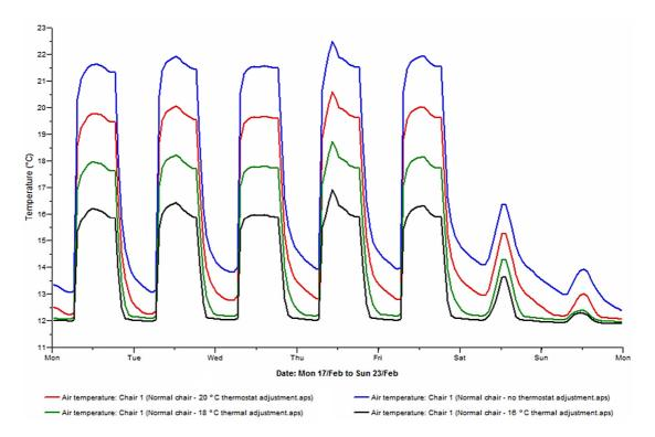
Figure 14. Air temperature results around the non heated chair when the setpoint was adjusted to 20, 18 and 16 °C ( $17^{th}$ - $23^{rd}$  February)
