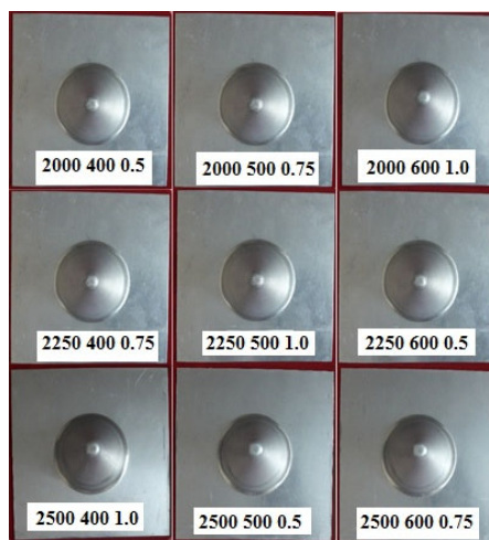
Fig. 4 Components formed as per L9 orthogonal array
